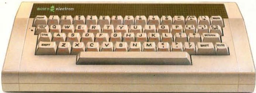
At the heart of the machine lies 64K of memory. Of this, 32K is in the form of ROM (Read Only Memory) containing the Machine Operating System and BASIC interpreter. The other 32K is RAM (Random Access Memory), over 20K of which can be available to you for writing your programs.
