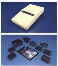
networks are joined together using Bridges. These provide high speed automatic connection between separate Econet networks. One of the advantages of joining networks together in this way is that if one section of the network fails, the rest of the Econet system is not affected.
