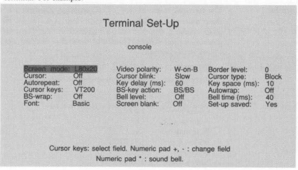
Pressing the <F3> key again will return to the original screen display, so that you can observe the effect of any changes. If you then press <F3> again, the set-up screen will reappear as you left it. You can switch between the set-up screen and the main display as often as you wish, until you are satisfied with your set-up.
