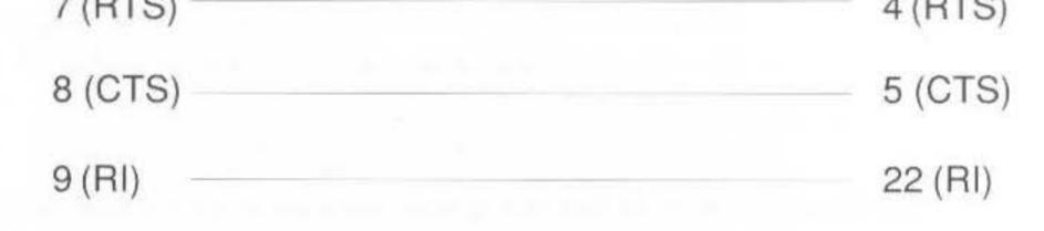
In practise you may leave out RI and DSR as they are not used. If the modem doesn't provide a CTS signal, leave out this wire and instead strap it to RTS at the RISC iX workstation end.
