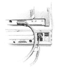
Finally, plug the connector on the mains cable into the socket marked I/P 220-240V on the back of the computer unit.
