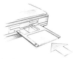
The disc clicks into place when it is fully inserted. Practise inserting one of the Applications discs.
