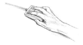
Move the mouse around and watch the pointer move around the screen. If you run out of space to move the mouse, lift it up and put it down again in a more convenient spot. While the mouse is lifted, the pointer will not move, and when you put it down again you can carry on where you left off.
