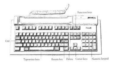
The keys are divided into blocks. The main block contains the keys similar to a typewriter keyboard. The Return key on the right completes a line, either starting a new line of text, or sending a name or instruction to the computer, depending on what you are doing.
