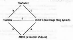
The names identify the component parts. The lines identify links between them:
