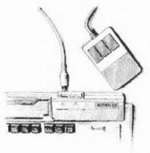
The keyboard has a curly cable with a plug on the end of it. Remove the red cover from the plug and push the plug into the socket on the front righthand side of the system unit (just below the disc drive slot), with the arrow uppermost. Don't force it. Place the keyboard in front of the computer.
