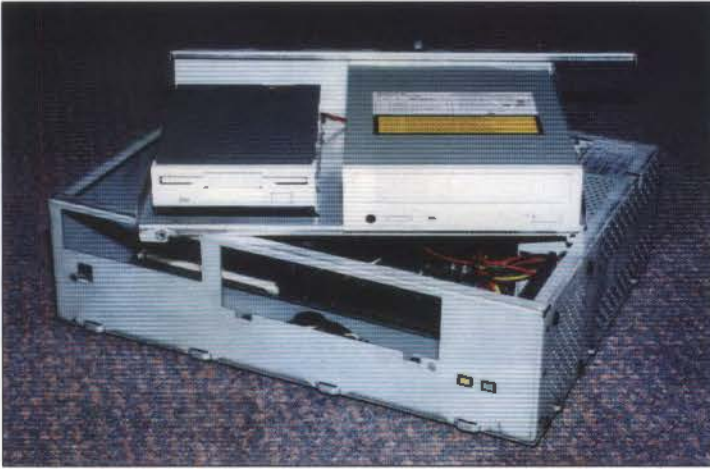
The A7000's drive mounting bracket is similar to that found in the old A5000.
