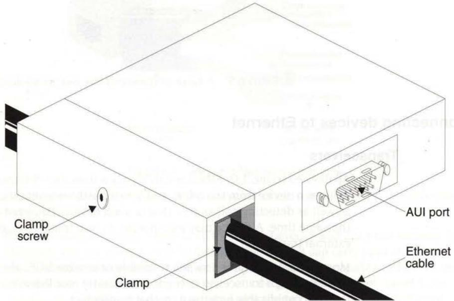
Figure 6.6 A thick Ethernet transceiver
