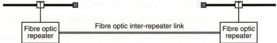
Figure 7.1 Connecting two Ethernet segments with a fibre optic inter-repeater link
