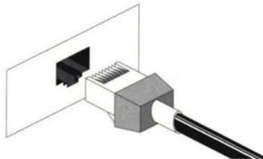
Figure 6.9 An RJ45 socket and lead
