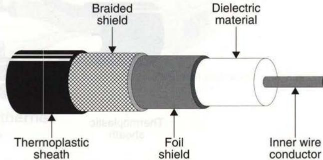
Figure 6.3 A coaxial cable
