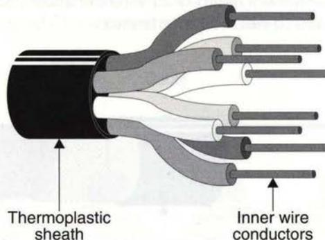
Figure 6.4 An unshielded twisted-pair cable
