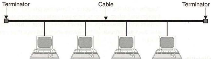
Figure 6.1 Bus topology, as used by thick and thin Ethernet
